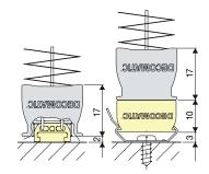
Reinforced profile – 17 mm. Includes bottom profile to embed the tension bracket.
